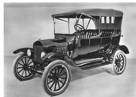
Vanadium steel was also used in the Model T Ford. Credit: Granger Historical Picture Archive / Alamy Stock Photo
